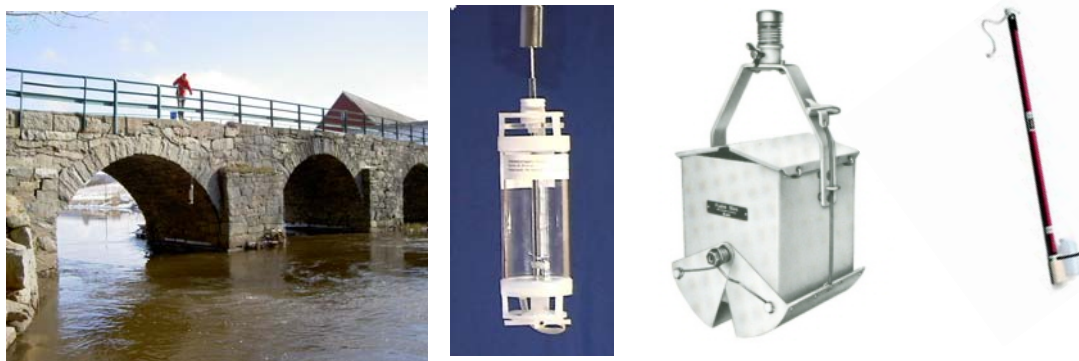
Figure 7. From left to right: Collecting water with Ruttner at Åsbro sampling point, Ruttner water sampler [92], Ekman grab sampler [92] and water collector for open waters [92].
